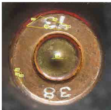
Figure 3.5.6 — View of the measurement results of linear parameters, traces of the strikers, reflector, shutter dosylatelya cartridge sleeve 9×18Mak, shot from a pistol IZH-70-18ME
